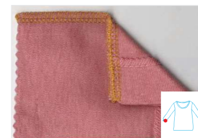
Four threads back latching stitch P17
