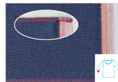
Three threads back latching stitch P17
