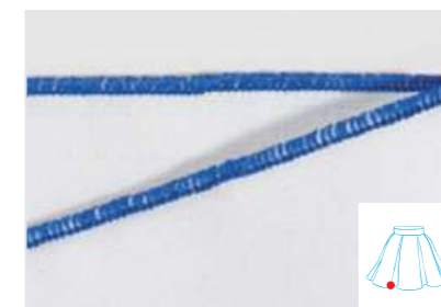
Three threads baby overlock stitch P15
