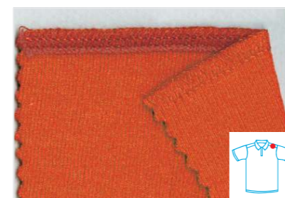
Four thread tape attach stitch P15
